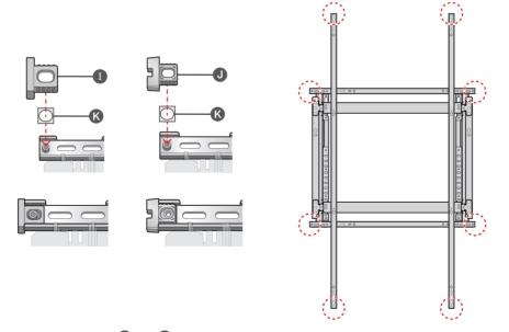
Use the tape K to attach the components 1 and 3, according to the specifications for your Signage model.
