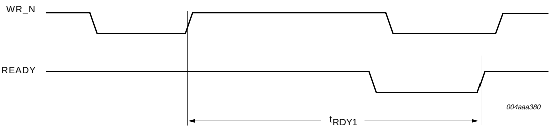
Fig 22. ISP1583 READY signal timing.
