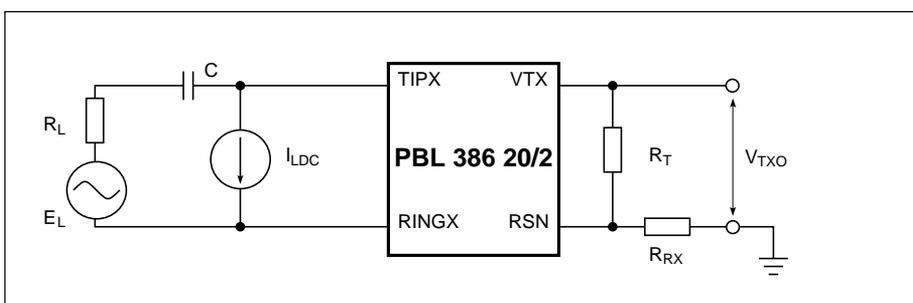
Figure 5. Overload level,  $V_{TXO}$ , four-wire transmit port
