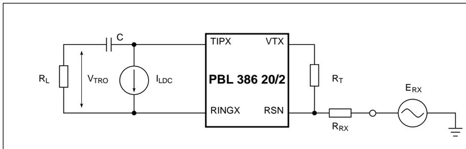
Figure 3. Longitudinal to metallic (B<sub>LME</sub>) and Longitudinal to four-wire (B<sub>LFE</sub>) balance
