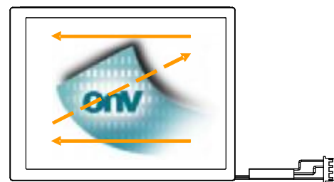
Fig. 2 Reverse scan (Pin19 = High)
