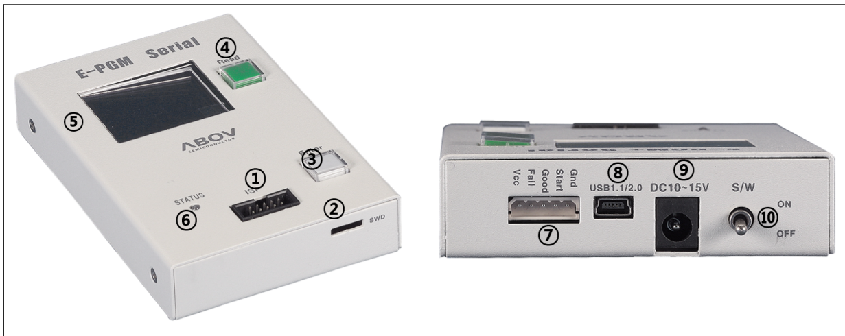
Figure 7: E-PGM Serial top and side views for function description
