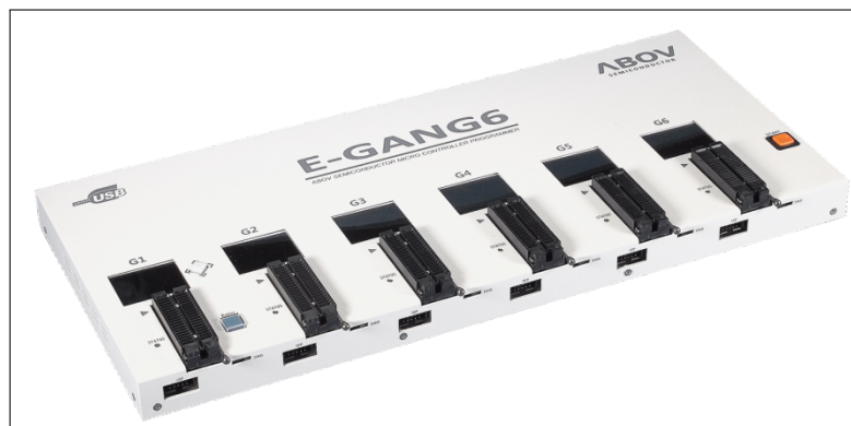
Figure 4: E-GANG6 exterior view
