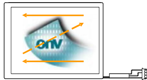
Fig. 2 Reverse scan (Pin19 = High)
