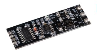
This UART TTL to RS485 converter allows you to add an RS485 interface to your single board computer.
