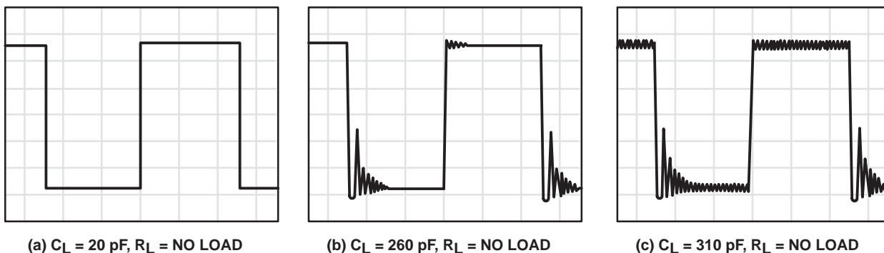
Figure 112. Effect of Capacitive Loads in Low-Bias Mode
