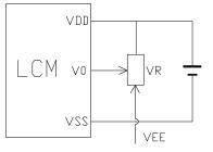
V<sub>DD-</sub>V<sub>0</sub>: LCD Driving voltage VR: 10k~20k
